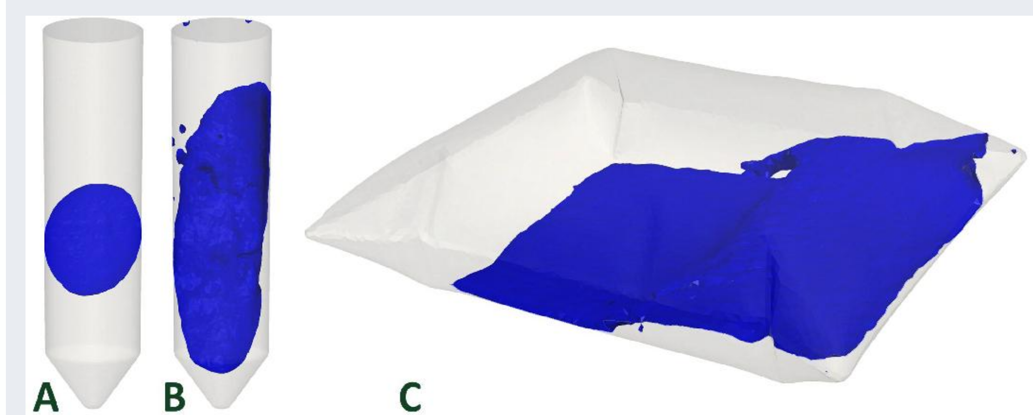
Figure 4: Surface of the TubeSpin with 20 mL filling volume, 50 mm amplitude, 150 rpm (A) and 240 rpm (B) and the orbitally shaken bag with 1 L filling volume, 50 mm amplitude, 40 rpm (C).
